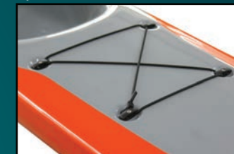
Deck rigging for accessible stowage.
