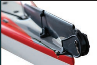
Smart-Track Over-Stern rudders systems with rudder keep.
