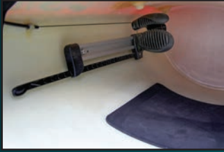
Smart-Track Transitional footbrace w/Toe pilot on steering boats.
