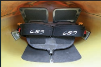
S18R/ST21: 3-point Quick-release carbon touring footbrace.
