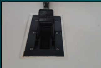
Quick draining DeBrito Bailer (Dual Venturi & Bullet Optional)
