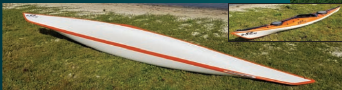
Keel Strip ( fiberglass or Kevlar, topped w/ Gelcoat)
