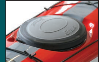
Large and Small oval water tight hatches with sealed bulkheads.
